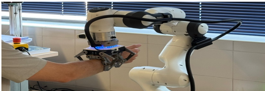
Instrumented underactuated gripper grasping a person's forearm.
