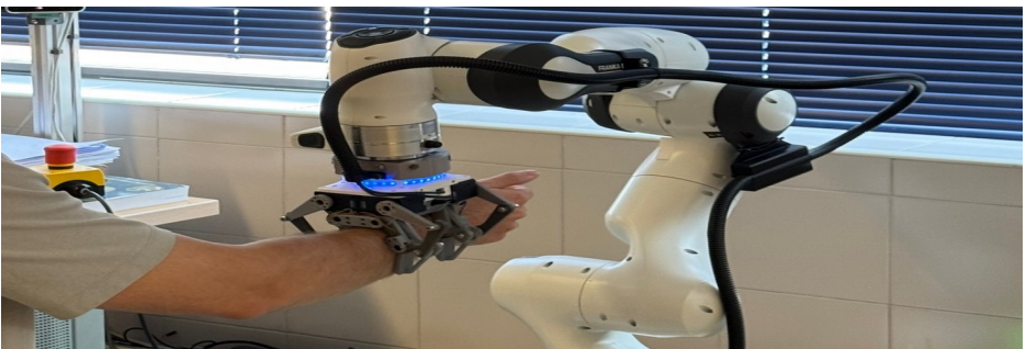
Instrumented underactuated gripper grasping a person's forearm.
